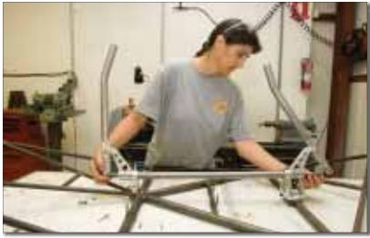
Weight-saving measures are being explored for both the SLSA and Experimental versions. This aluminum control-stick setup could trim a few pounds.
