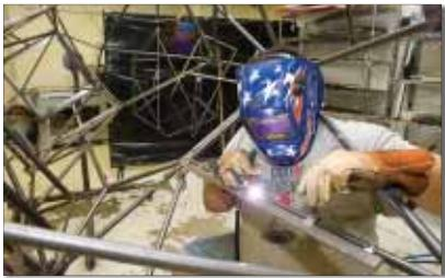
After primary jiggling, the Cub's frame is TIG welded.
