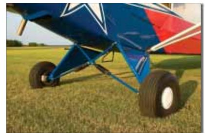
Look, Mom: No bungee cords. Small springs are mounted in line with the main-gear tension struts.
