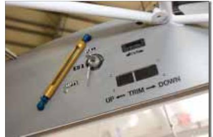
Above the pilot's head are simple sight gauges for fuel quantity, the ignition switch and a big-as-life trim indicator.
